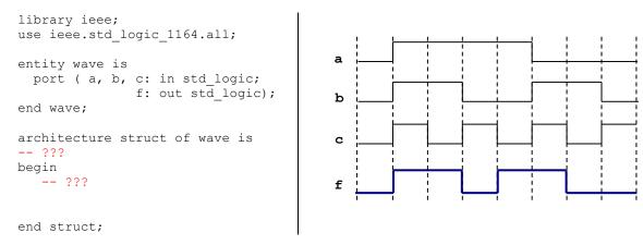
b) Complete the timing diagram of the logic circuit whose VHDL description is shown below: (5 pts)
